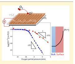
a lower effective defect formation energy at the surface region compared with that in the bulk. In addition, the  $Pr^{3+}$  concentration has a weaker dependence on  $pO_2$  compared to that in the bulk.
