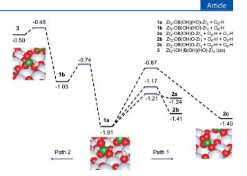
**Figure 8.** Potential energy diagram of  $B(OH)_3$  on  $ZrO_2(\overline{1}11)$  showing the energy barriers for two reaction pathways, further dissociation of the single O–H dissociated structure into double O–H dissociated structures (Path 1), and transition from a single O–H dissociated structure to a cis-molecular adsorption configuration (Path 2).
