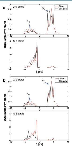
**Figure 6.** Projected density of states (PDOS) for the surface Zr and O atoms, obtained in the case of the most stable molecular adsorption (a) and dissociative adsorption (b). The states for the clean and adatom sites are marked in red and black, respectively.
