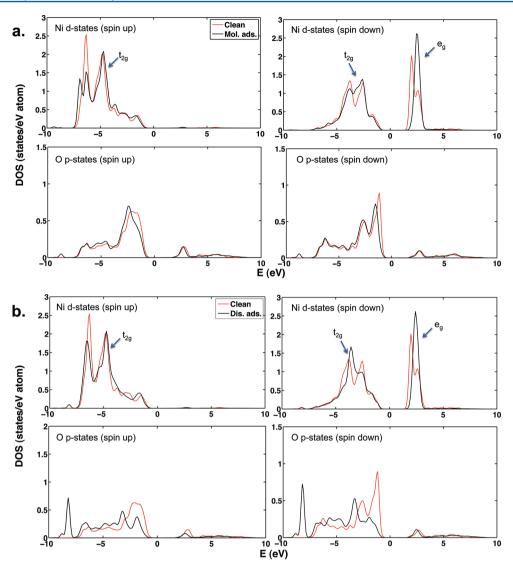
Figure 5. Projected density of states (PDOS) for the surface Ni and O atoms, obtained in the case of the most stable molecular adsorption (a) and dissociative adsorption (b). The states for the clean and adatom sites are marked in red and black, respectively.
