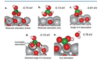
**Figure 3.** Reaction sequence showing the most favorable molecular and dissociated adsorption configurations of  $B(OH)_3$  on NiO(001), and the corresponding adsorption energy values. Note that the double O–H bond dissociation is unstable, and we obtain a distorted single O–H dissociated structure. The arrows in black indicate dissociation.
