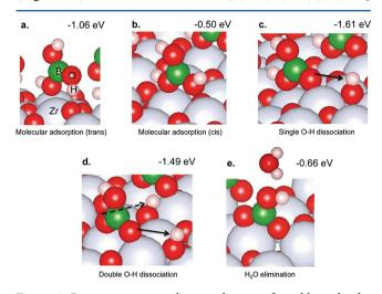
**Figure 4.** Reaction sequence showing the most favorable molecular and dissociated adsorption configurations of  $B(OH)_3$  on  $ZrO_2(\overline{1}11)$ , and the corresponding adsorption energy values. The arrows in black indicate dissociation.
