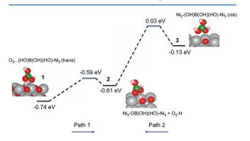
**Figure 7.** Potential energy diagram showing the reaction energy barriers for single O–H dissociation of  $B(OH)_3$  on NiO(001), starting from the trans-molecular configuration (Path 1) and cis-molecular configuration (Path 2).
