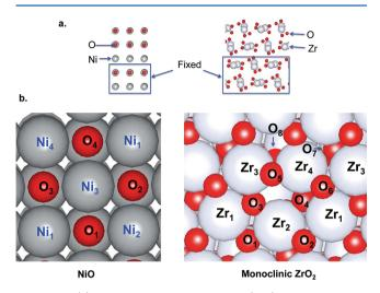
**Figure 1.** (a) Slab models used for NiO(001) and monoclinic  $ZrO_2(\overline{1}11)$  surfaces. (b) Top view of the NiO(001) and monoclinic  $ZrO_2(\overline{1}11)$  surfaces. The NiO surface unit cell chosen consists of four Ni and O atoms, while the  $ZrO_2$  surface unit cell consists of four Zr and eight O atoms. The numbering scheme is used to characterize adsorption structures later.
