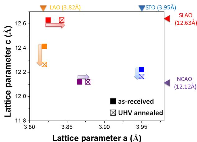
Figure 3. Change of the out-of-plane lattice parameter of NNO films on various substrates upon annealing in UHV conditions at 700 °C.
